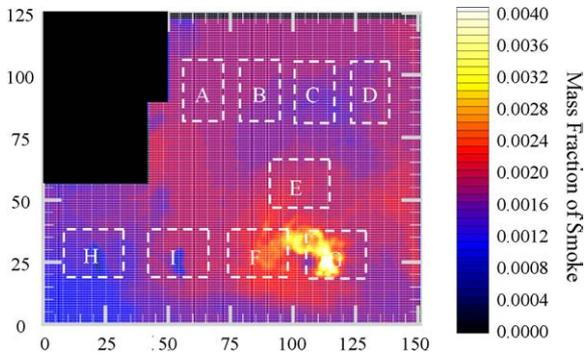
Fig. 4. FDS steady smoke concentration distribution and zone layout (spatial dimensions are in meters).
